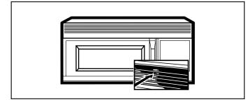
3. Remove 2 screws located above door near center of oven. Remove light bulb cover.
